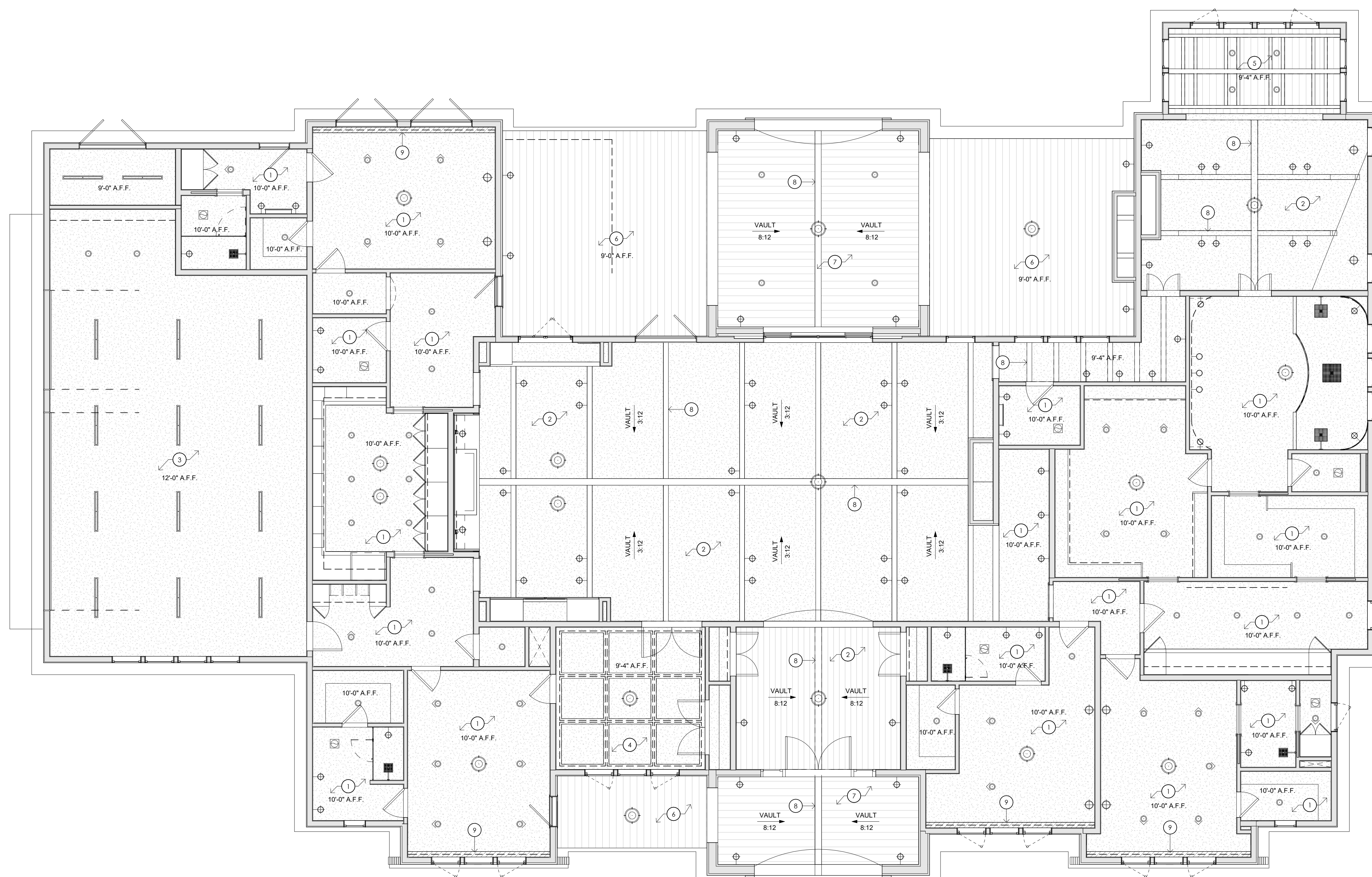
1 FIRST FLOOR REFLECTED CEILING PLAN 3/16" = 1'-0"
